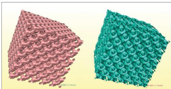
**Figure 2:** Highest Occupied Molecular Orbital (right) and Lowest Unoccupied Molecular Orbital (left) of a silicon supercell containing 1000 atoms. The ability to study such large structures is important for modeling defects, fracturing, and dopants at low concentrations
