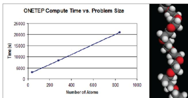
**Figure 1:** ONETEP linear scaling behavior for the calculation of the total energy for a polyethylene oxide (PEO) polymer chain. Calculation run on 16 dual-core Opteron 2.8 GHz processors, 1 MB cache, 8 GB per processor.
